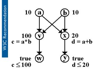
Vertices a and b have edges leading to v and x because these vertices represent the calculate expressions of c and d, which reference a and b to compute their product and sum, respectively. Similarly, v and x have directed edges to w and y, respectively, because w and y represent the constraint expressions of c and d, which reference the values of c and d to compare them with boundary values.
